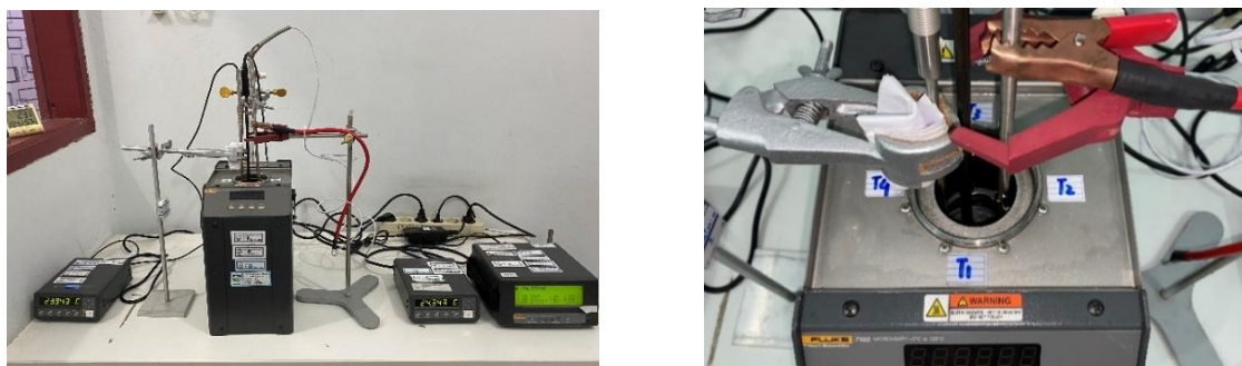
Figure 3 - Microbath homogeneity and stability test process
