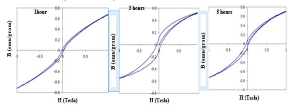
**Figure 2.** Hysteresis curve of the BaFe<sub>12</sub>O<sub>19</sub> wich was sintered at 300<sup>0</sup>C
