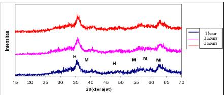
**Figure 1**. X-ray diffraction patterns of samples sintered at 300°C with various holding times of 1 hour, 3 hours and 5 hours.
