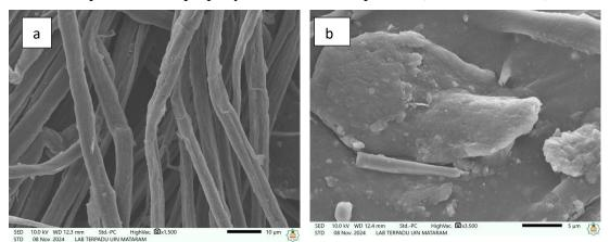
Figure 3. SEM Images of Treated PALF
