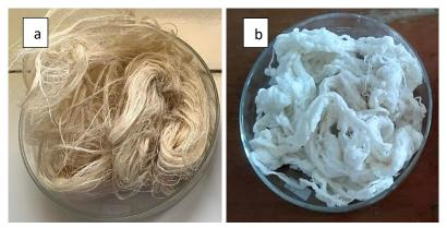
Figure 1. The Untreated PALF (a) Treated PALF (b)
