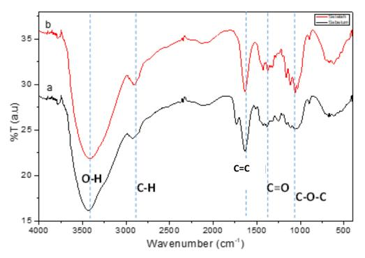
Figure 2. FTIR Spectra of Treated and Untreated PALF
