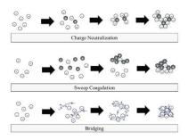
Figure 2. Coagulation Process
