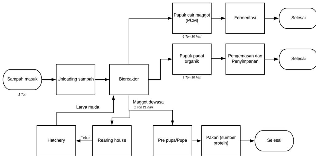
**Gambar 2. Diagram alir operasional BSF**
