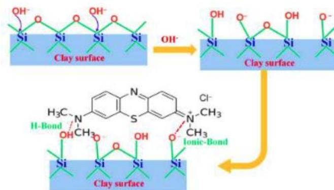
Figure 2. Interaction of clay molecules and blue methylene dye in alkaline pH.
