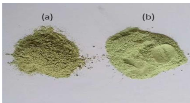
Figure 2. (a) Natural zeolite and (b) Activated natural zeolite
