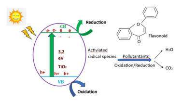
Figure 6. Photocatalytic mechanism of TiO2 nanoparticles under light
