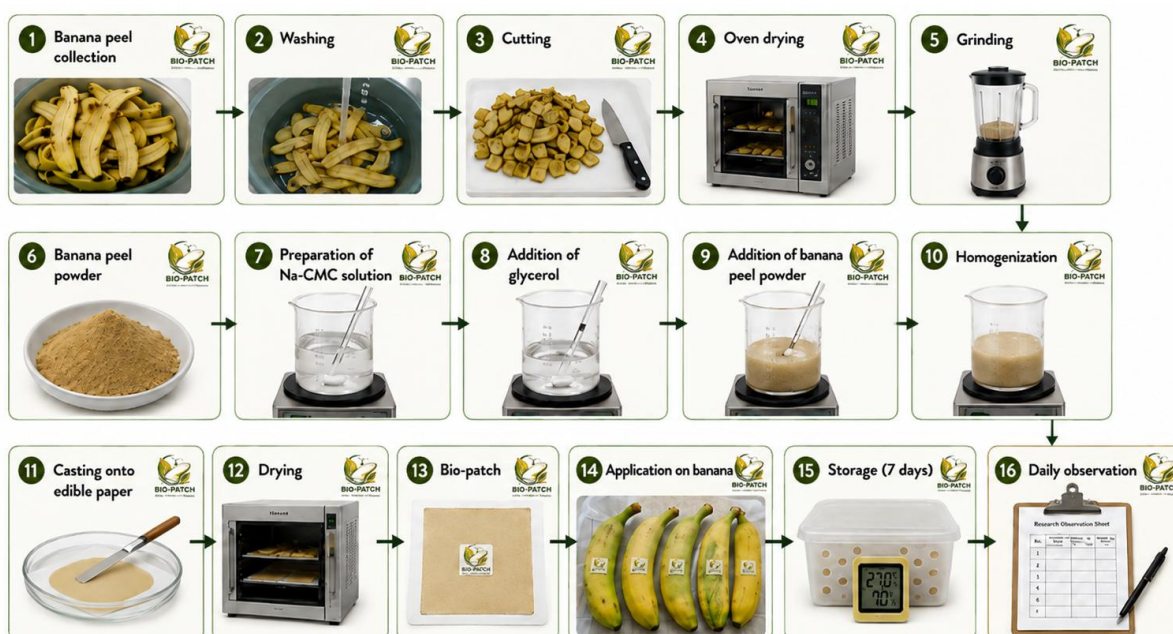
Figure 1. Flowchart of the experimental procedure
